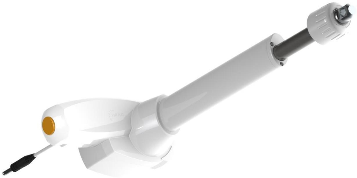
RE708 is a compact and very efficient, 8kN actuator developed to meet the requirements in patient lifts. It is equipped with a manual lowering function, which allows lowering the lift by hand if the electrical power is not available. It also has a pull force protection to prevent injuries.
