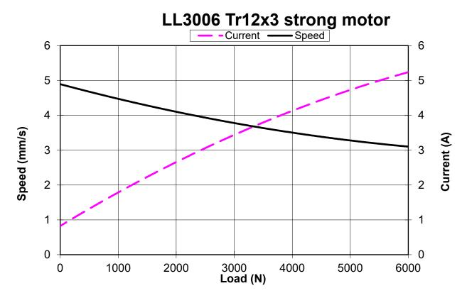
Charts show average figures for 24V actuator using stabilized power supply. Figures all with ambient temperature of 20°C. Accuracy: ±5
