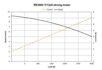
Charts show average figures for 24V actuator using stabilized power supply. All figures with ambient temperature of 20°C. Accuracy: ±5.
